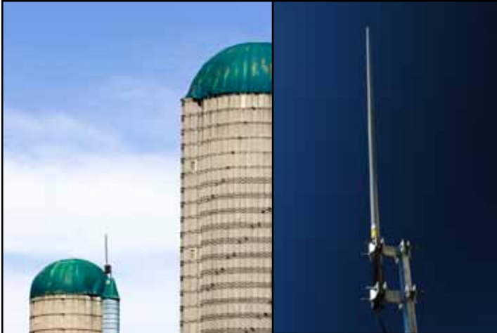
Base station high gain omnidirectional antennas collect data from the rovers and assist in differential correction for precision agriculture.
